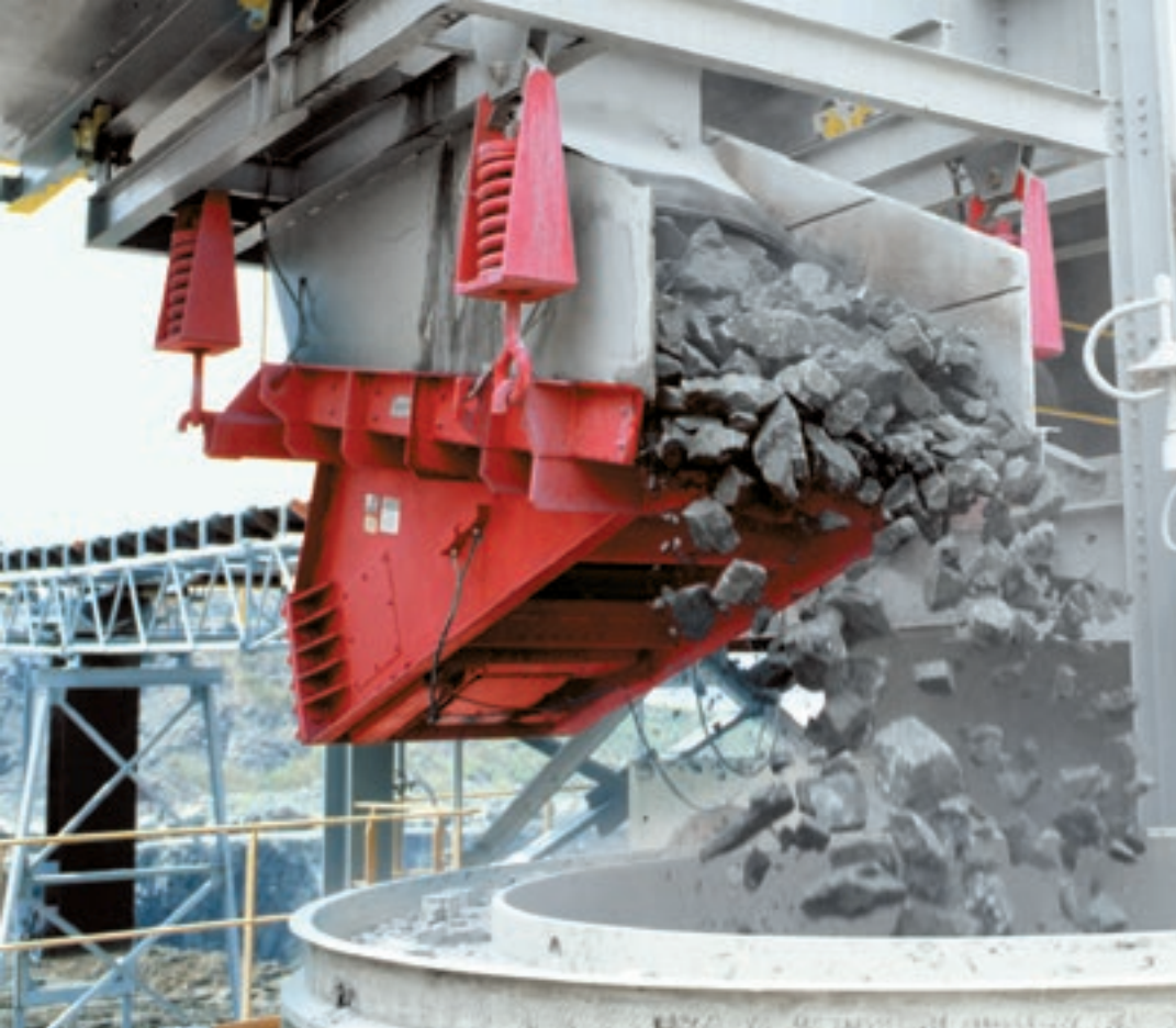
Syntron® MF-600 Electromechanical Feeder feeding rock to a crusher.
