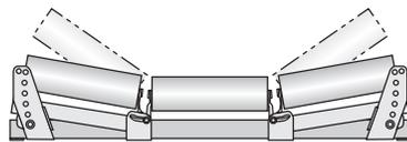
**Variable troughed belt idlers** placed between the final troughing idler and the head pulley, support the belt during its transition from a concave to a flat contour. The end rolls can be adjusted vertically to match the changing contour of the belt during this critical period of transition.
