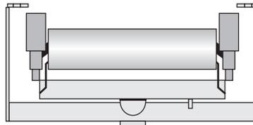
**Return belt training idlers** train the belt and protect its edges from damage caused by misalignment. Positive action type for belts operating in one direction. Actuating shoe type for reversing belts.
