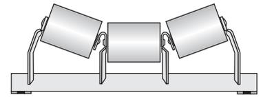
**Troughed belt idlers** for general carrying service are available with roll inclinations of 20°, 35°, and 45°.
