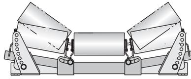
**Variable troughed belt idlers** placed between the final troughing idler and the head pulley, support the belt during its transition from a concave to a flat contour. The end rolls can be adjusted vertically to match the changing contour of the belt during this critical period of transition. Standard design features steel rolls. Also available with all rubber cushion rolls or rubber cushion center roll and steel end rolls.
