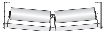
**Rigid frame v-return idlers** provide a means of training the return belt, with the added benefit of additional carrying load capacity. Rigid v-returns can be adjusted using slotted bolt holes in the end brackets of the frame to aid in proper belt training.
