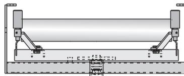
**Return belt training idlers** train the belt and protect its edges from damage caused by misalignment. Positive action type for belts operating in one direction. Actuating shoe type for reversing belts.
