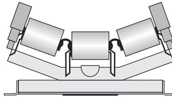
**Troughed belt training idlers** automatically train belts and protect belt edges from damage caused by misalignment. Positive action type available for belts operating in one direction, and actuating shoe type available for two-directional operation (reversing).
