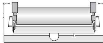
**Return belt training idlers** train the belt and protect its edges from damage caused by misalignment. Positive action type for belts operating in one direction. Actuating shoe type for reversing belts.
