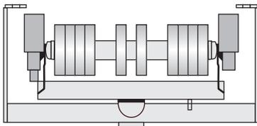
**Return rubber tread training idlers** train the belt and protect its edges from damage caused by misalignment. Used when wet or sticky materials tend to cling to the belt, where corrosion resistance is required or where chemical reaction to iron or steel is involved. Positive action type for belts operating in one direction. Actuating shoe type for reversing belts.
