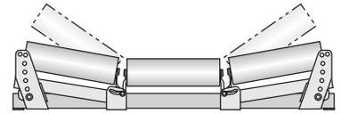
**Variable troughed belt idlers** placed between the final troughing idler and the head pulley, support the belt during its transition from a concave to a flat contour. The end rolls can be adjusted vertically to match the changing contour of the belt during this critical period of transition.
