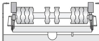
**Return rubber tread training idlers** train the belt and protect its edges from damage caused by misalignment. Used when wet or sticky materials tend to cling to the belt, where corrosion resistance is required or where chemical reaction to iron or steel is involved. Positive action type for belts operating in one direction. Actuating shoe type for reversing belts.
