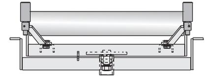
**Flat belt training idlers** automatically train belts and protect belt edges from damage caused by misalignment. Available in the positive action type for belts operating in one direction.
