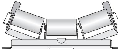
**Troughed belt training idlers** automatically train belts and protect belt edges from damage caused by misalignment. Positive action type available for belts operating in one direction, and actuating shoe type available for two-directional operation (reversing).
