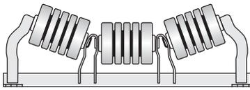
**Troughed belt rubber cushion idlers** protect the belt by absorbing impacts at loading and transfer points. Design features include removable end brackets on 35° and 45° idlers.
