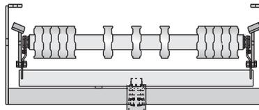
**Return rubber tread training idlers** train the belt and protect its edges from damage caused by misalignment. Used when wet or sticky materials tend to cling to the belt, where corrosion resistance is required or where chemical attraction to iron or steel is involved. Positive action type for belts operating in one direction. Actuating shoe type for reversing belts.
