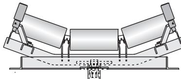
**Troughed belt training idlers** automatically train belts and protect belt edges from damage caused by misalignment. Positive action type for belts operating in one direction; actuating shoe type for two directional operation (reversing).
