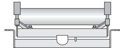
**Flat belt training idlers** automatically train belts and protect belt edges from damage caused by misalignment. Available in the positive action type for belts operating in one direction.
