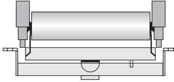
**Flat belt training idlers** automatically train belts and protect belt edges from damage caused by misalignment. Available in the positive action type for belts operating in one direction.
