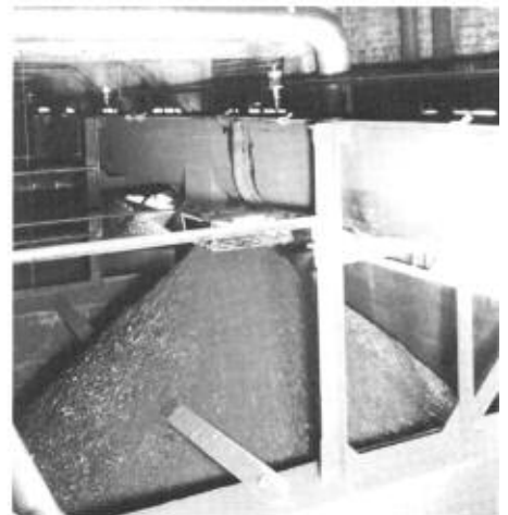
Top Right - Over 40 feet of screw conveyors carry malt and rice from storage to mills in this factory.
