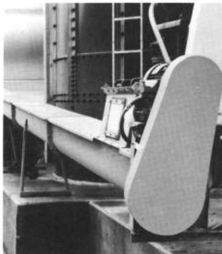
Bottom Left: Heavy-duty sectional flight conveyor augers installed on boring machine.
