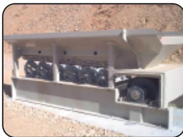
A tail loading section has the same features as the tail section plus the addition of an integral loading section.
