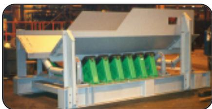
Syntron Material Handling offers Link-Belt® intermediate loading sections for all transition angles, with associated chute and skirt arrangements.
