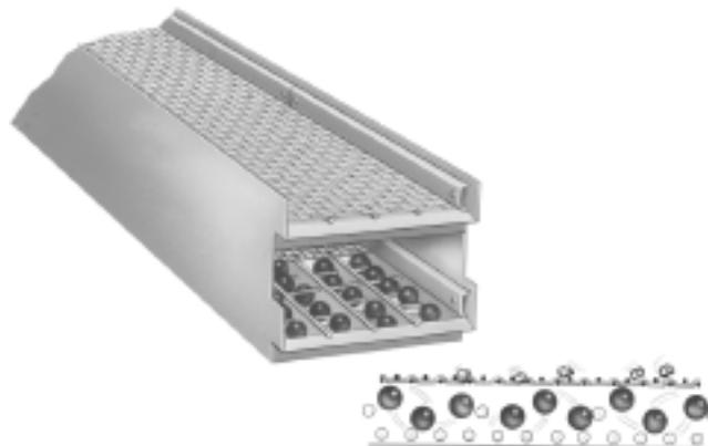
Electrically heated screen cloth can be used on Syntron Material Handling vibrating screens to prevent screen cloth blinding due to fine particles accumulating on the wires when handling sticky or hygroscopic materials. Screen cloth tensioning devices facilitate the flow of electricity from transformer to screen cloth, providing uniform heating with very low current consumption.
