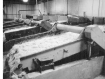
Four Link-Belt® Model NRM liquid Vibrating screens dewatering feathers and offal in a chicken processing plant.
